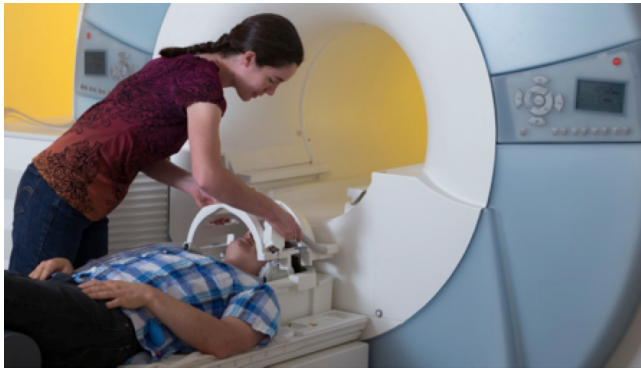
Figure 1. The fMRI scanner. A volume coil (with mirror to view the computer monitor) is placed over the participant's head.
